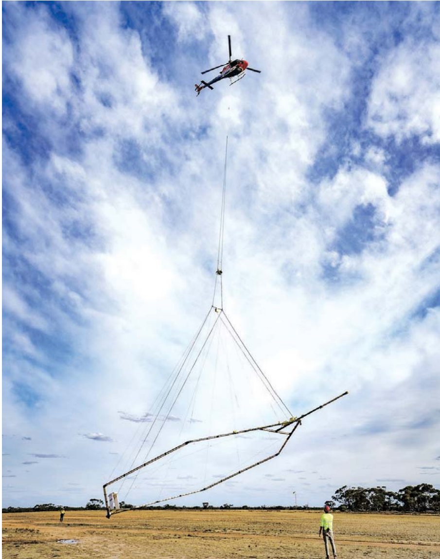
The helicopter carrying transmitter and receiver coil is in the area undertaking research into dryland salinity.
